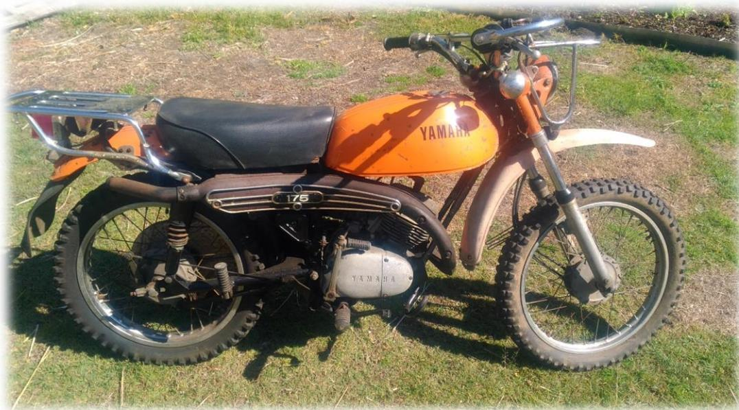
They were simple in design but developed after extensive testing. A basic single cylinder two stroke with auto lube (Yamaha's automatic oil in
